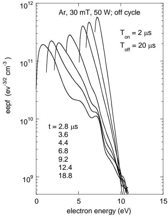
**Fig. 2.** The EEPF evolution in the afterglow stage. EEPFs are shown in order from left to right as the elapsed time,  $t$ . The shift in the EEPF position along the energy axis corresponds to the plasma potential shift, reference to the plasma potential at  $t = 2.8 \mu\text{s}$ .
