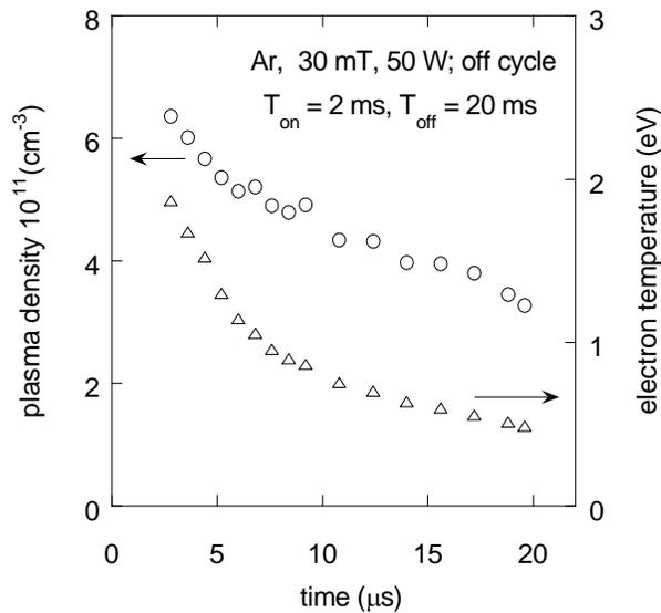
**Fig. 3.** Plasma parameters in the afterglow stage. By the end of the afterglow period, the electron temperature is an order of magnitude less than that in the CW mode. Due to absence of the electric field and reduced electron temperature, the EEPF in the late afterglow stage is Maxwellian.
