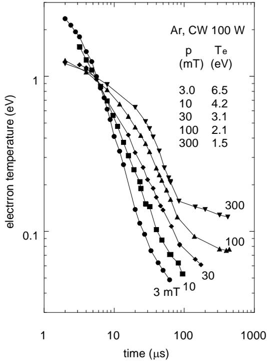
**Fig. 1.** T<sub>e</sub> in the CW mode (table) and the EEPF in the afterglow
